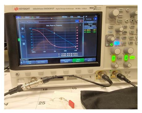
The Function Generator and the Ch1 input have been connected together with a T connector. If no T connector is available use seperate BNC to gator connectors. Connect the internal Function Generator output of the scope to the input of the circuit and the Ch 1 input to the input of the circuit. Also connect Ch2 of the scope to the output of the circuit. The Bode Plot shown is for a first order passive low pass filter. The cursons have been move to the - 3dB filter.
