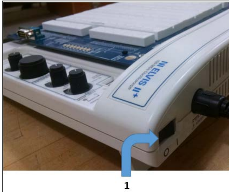
Fig.5 Location of NI ELVIS II + general turn on button.
