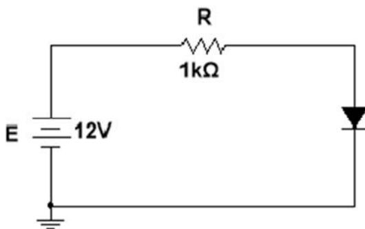
Figure 11.18: Circuit for Determining Diode Parameters.
