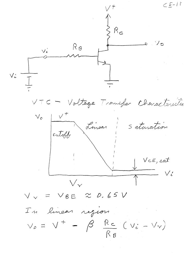
Common Emitter Amplifier For design calculations tie + Rte
