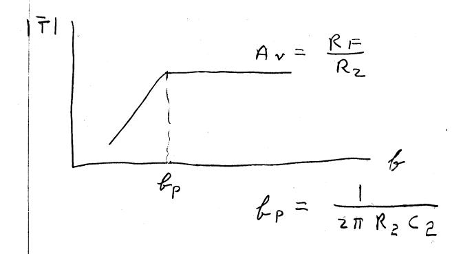
Non I deal Op Amp Finite Lecin Finte Bandwidth -Peak Clipping Output Rurrent Limiting 5 lew Rate Limiting I nput Bias Currents DC Officet
