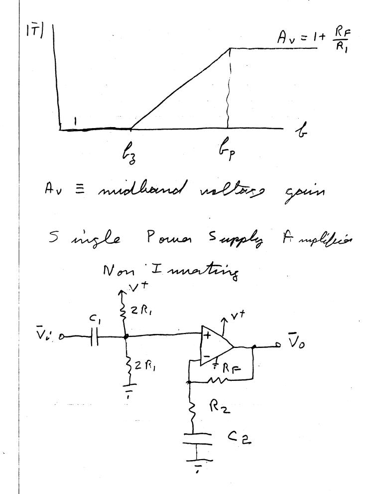
$$T = \frac{V_0}{V_i} = \frac{2R_1C_1}{1 + 2R_1C_1} \left[ 1 + \frac{R_F}{R_2 + \frac{1}{2c_2}} \right]$$
