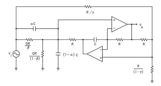
$$T(s) = \left[ \frac{\left(\frac{s}{\omega_o}\right)^2 \cdot (2 \cdot \alpha - \gamma) + \frac{1}{Q} \cdot \left(\frac{s}{\omega_o}\right) \cdot (2 \cdot \beta - \gamma) + \gamma}{\left(\frac{s}{\omega_o}\right)^2 + \frac{1}{Q} \cdot \frac{s}{\omega_o} + 1} \right]$$
