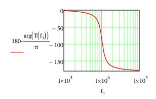
Third Order Elliptic Filter with 0.5 db ripple unity dc gain with stop band to cutoff ratio of 1.5
