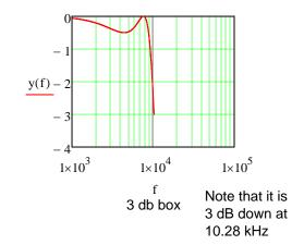
Now the circuit must be designed. This requires a 1st order lpf cascaded with a 3rd order lpf. This can be done by cascading the circuit shown in Fig. 6.9.a (page 83) with Fig. 6.11 (page 83).
