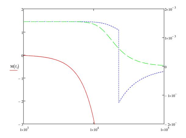
$$n = 3 \qquad \qquad \frac{f_3}{f_c} = 1.7557 \qquad a_1 := 2.5415 \\ a_2 := 2.3222 \\ T(s) = \frac{1}{\frac{s}{a_2 \cdot \omega_c} + 1} \cdot \frac{1}{\left(\frac{s}{a_1 \cdot \omega_c}\right)^2 + \frac{1}{b_1} \cdot \frac{s}{a_1 \cdot \omega_c} + 1} \qquad \qquad \text{1st Order LPF}$$
