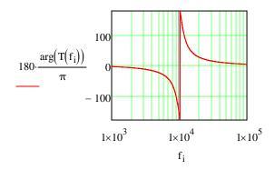
Notch  $\alpha := 1$   $\beta := 0.5$   $\gamma := 1$  Q := 3  $f_0 := 10.28 \text{kHz}$
